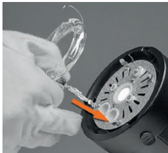
Fig. 2: To insert a new flash tube, support the legs of the flash tube and carefully push the flash tube into the end position. Then wrap the ignition wire around the flash tube holder again.
