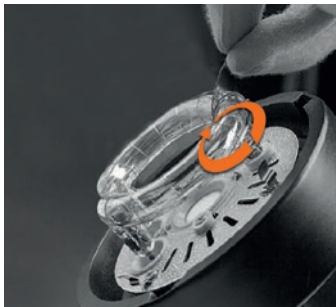
Fig. 1: Unwind the twisted ignition wire from the flash tube holder and carefully pull the flash tube out of the unit.
