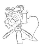
Attach a DSLM camera onto the tripod by using the 1/4 inch thread of your camera.
