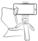
Furthermore you can connect the LED light within the USB slot of the tripod, to increase the light situation of your photo.
