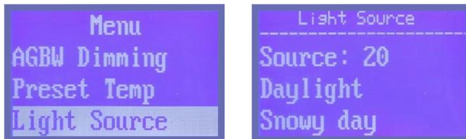
Instead of manually setting the color temperature of the LED lights, you can also use different scene modes.
