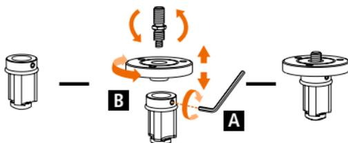
To use the tripod in the lowest position please use the short center column. It provides 360 degrees horizontal and 180 degrees vertical adjustments.
