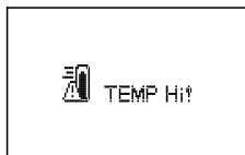
Flash high temperature alarm
